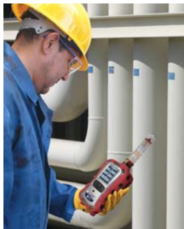
Multi RAE Benzene used for leak detection
