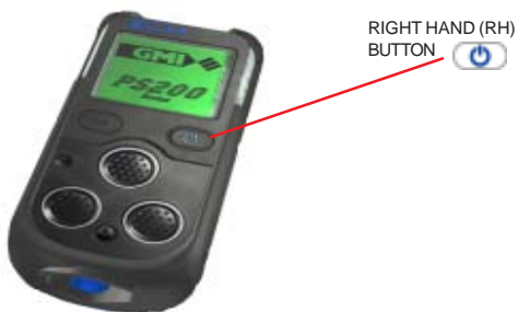
Fig. 2-1 PS200 Switch ON
