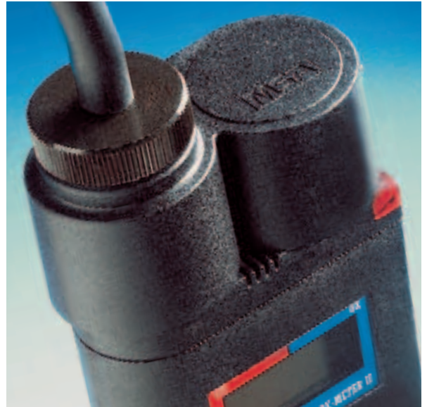
All EX-METER II and EX-OX-METER II instruments can be supplied with an integrated pump. The sampling is by diffusion; with the pumped version the attachment of a pump adapter [see above] permits sampling with an electric pump, sampling line and probe.
